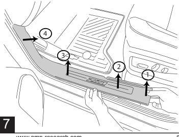
Pull up the carpet and drill 9/32" hole in metal and insert supplied rubber grommet (18).
