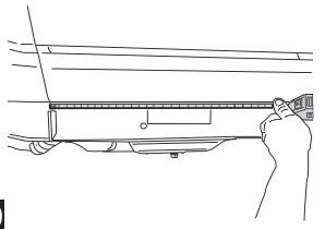
Affix lamp to rocker panel surface. Make sure the lamp is affixed to a clean, flat surface. There is a step down midway across the surface. Affix lamp just outside of step down.
