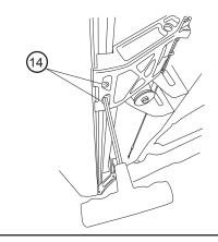
Using the two 11" cable ties, mount controller to support arm next to battery. Plug in harness (Ensure that locking tabs engage)
