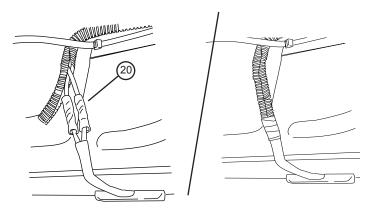
Connect harness to motor. Secure harness with tie wraps.
