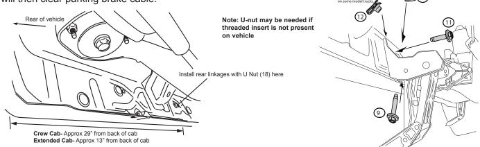
Set linkage into second to last sheetmetal tab / hole from rear. Use supplied bolt (9) and nut(10) to hold in position. Install bolt (11) into upper mounting hole and snug both bolts. Torque upper bolt (11) to 16ft-lbs(22N m) first and then torque lower bolt (9) and nut (10) to 16 ft-lb (22N m). Repeat linkage installation on Passenger side.
